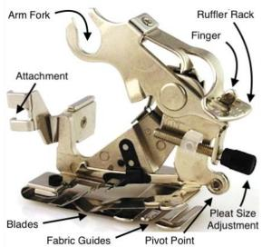
**Pleat Size Adjustment -** Determines the depth of the little pleats. There are several different models. Just look for a small screw that adjusts in and out.
